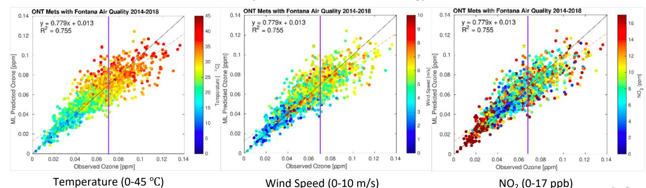
During peak ozone hours (12:00 – 5:00 PM), high ozone is associated with high temperatures, moderate wind speeds, and lower NO<sub>2</sub>
