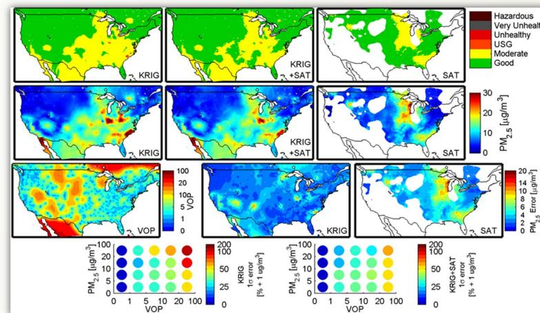
Kriged (KRIG), combined (KRIG+SAT), and satellite-derived (SAT) air quality index (first row); PM<sub>2.5</sub> concentrations (second row); variance of prediction (third row); and observed error as a function of PM<sub>2.5</sub> concentrations and VOP for the kriged and combined surface for July 1, 2011 (fourth row).
