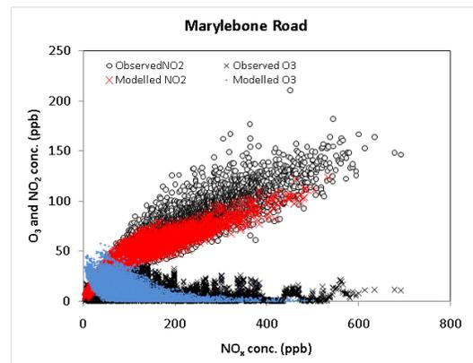
Fig. 2. Observed and modeled NO<sub>2</sub>, O<sub>3</sub> and NO<sub>x</sub> relationship at Marylebone Road in 2006
