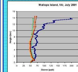
Ozonesonde data for Wallops Island, VA (average of sondes released on July 3, 11, 18 and 26) plotted with CMAQ predicted average ozone concentrations from the same days and times. All the simulations underestimate ozone above one kilometer, regardless of the vertical-layer structure or boundary conditions used.
