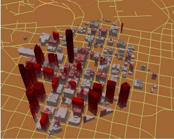
Fig. 1: Three-dimensional digital elevation data derived from an airborne lidar platform for a 1X1-km section of downtown Houston.
