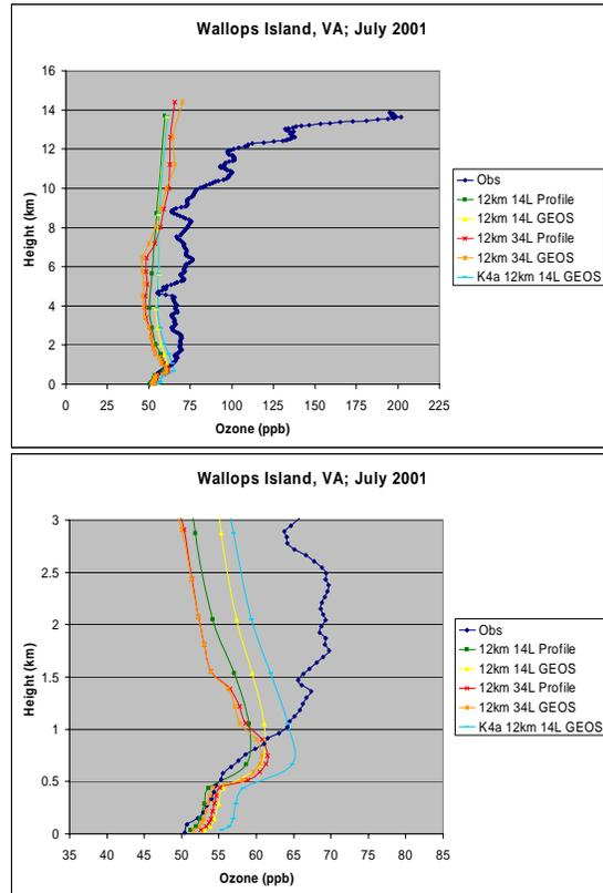
Figure 3. Ozonesonde data for Wallops Island, VA for July 2001 (average of sondes released on July 3, 11, 18 and 26) plotted along with vertical ozone concentrations from the various 12x12-km horizontal grid resolution sensitivity simulations.  $O_3$  concentration (ppb) is plotted along the ordinate and height (km) is plotted along the abscissa. The full extent of the model vertical profile is plotted above, while only the lowest 3 kilometers (roughly the boundary layer) is plotted below.
