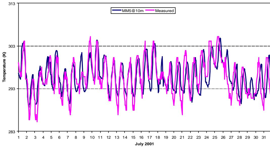
Figure 1. Temperature time series for MM5 predicted and monitored at the New Castle County Airport.
