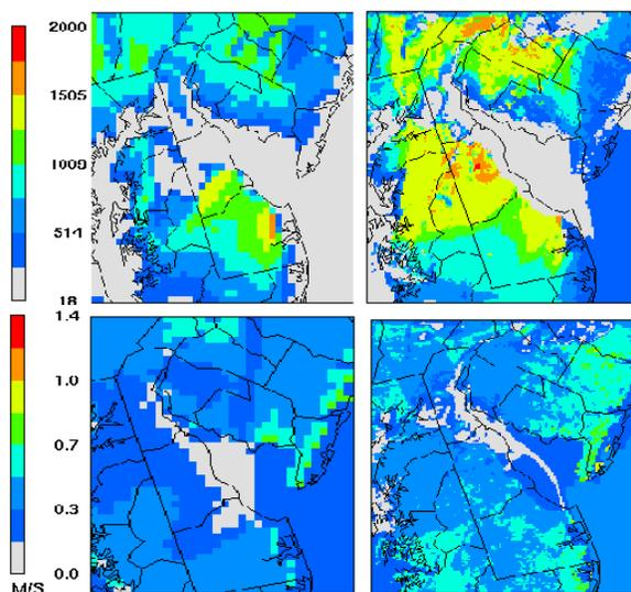
Figure 3. Dispersion parameters for July 4<sup>th</sup> 2001 at 6:00 pm EST: left side is 4-km grid; right side is 1-km grid. Top is PBL height (m); bottom is ustar (m/s).
