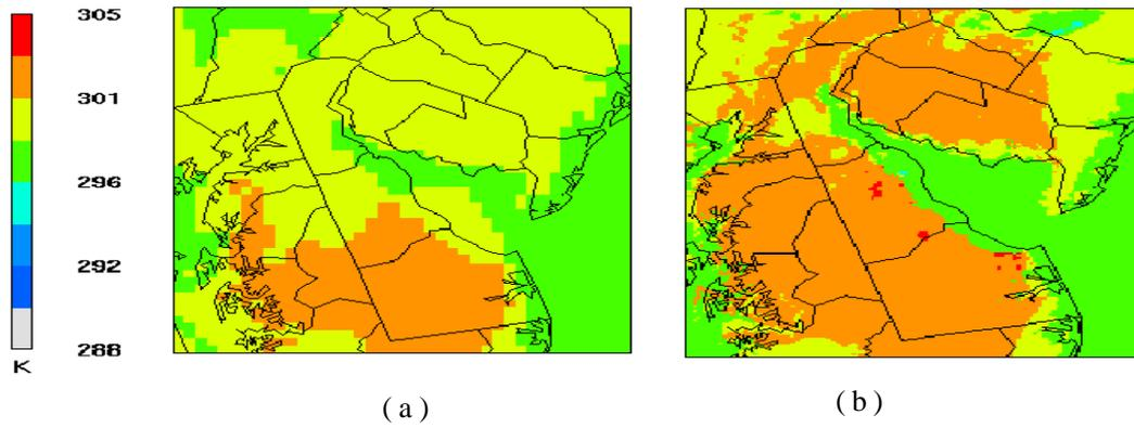
Figure 2. Temperature fields interpolated from MM5 layer 1 to 1.5 m for July 4<sup>th</sup> 2001 at 6:00 pm EST; left 4-km run and right 1-km run.
