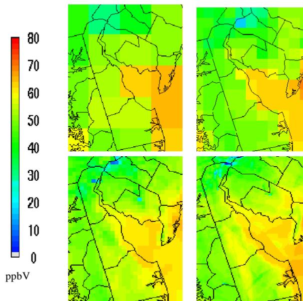
Figure 4. CMAQ-AT ozone simulation for July 2<sup>nd</sup> 2001 at 7:00 pm EST. Top (36-km and 12-km); bottom (4-km and 1-km).
