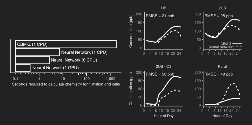
Left: Time required for one million independent simulations using either CBM-Z using one CPU core, the neural network using one or eight CPU cores, and the neural network using one GPU. Right: Comparisons of CBM-Z and neural network simulated diurnal O<sub>3</sub> concentrations for representative initial conditions.
