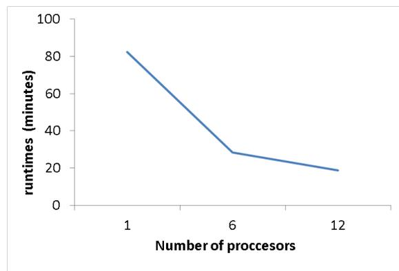
Fig. 2. Comparison of model runtimes for one day simulations for London against the number of processors
