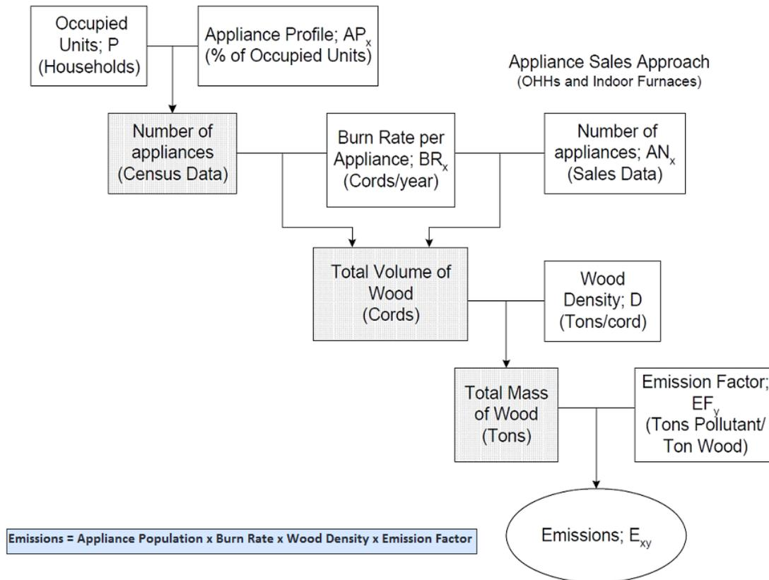
Figure 1. Data flow diagram for the RWC Tool.
