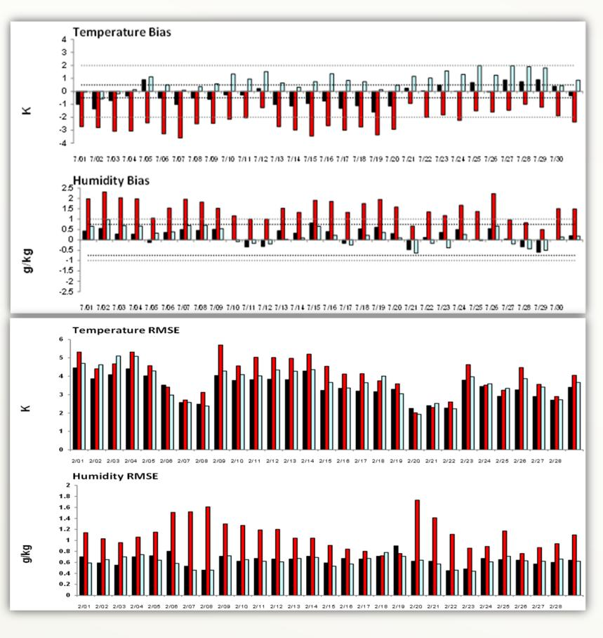
Daily temperature and humidity model performance for the LSM sensitivity experiments. The top two images show biases from the summer sensitivity, while the bottom two images show root mean square errors (RMSE) for the winter sensitivity.
