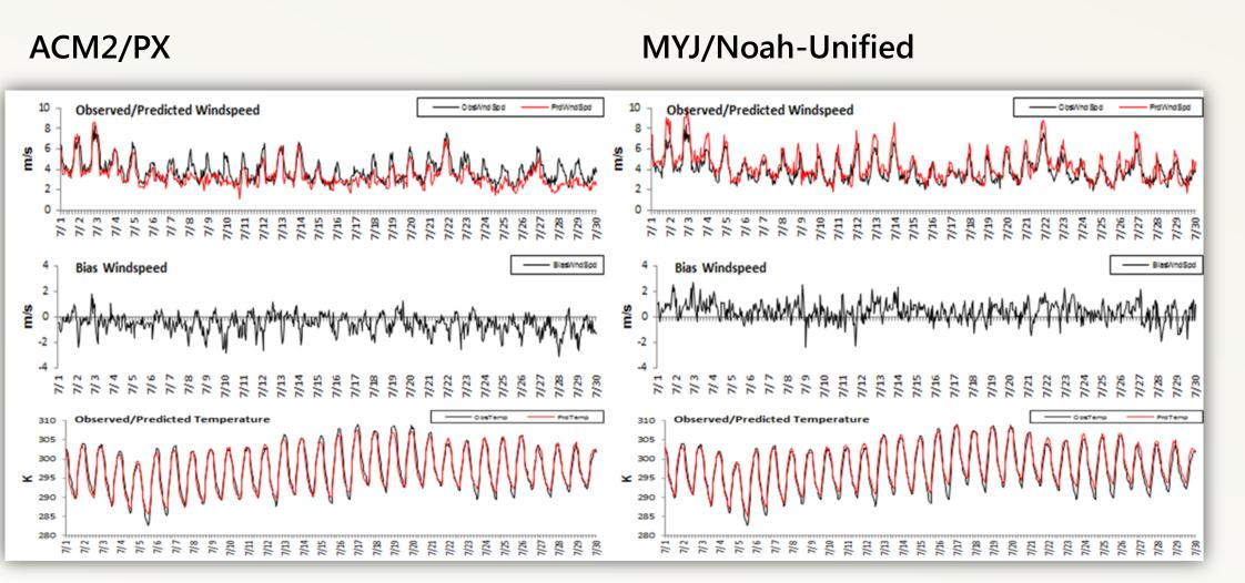
Observed (black) and predicted (red) wind speed, wind speed bias, and temperature for the summer sensitivity experiments for the WRF 4-km domain.
