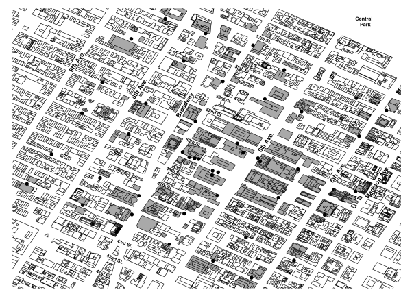
Figure 1. Building layer map of midtown Manhattan. Tracer gas measurement locations are marked with black dots, and buildings included in the models are highlighted in grey. The figure is oriented with north to the top.
