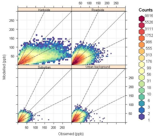
Fig. 3. Scatter plot of observed and modeled NO<sub>2</sub> concentrations at kerbside, roadside, urban background and suburban sites in 2006.
