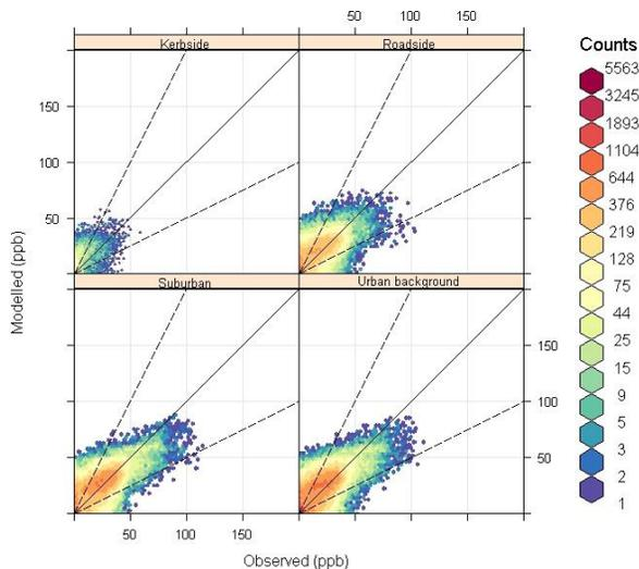
Fig. 4. Scatter plot of observed and modeled O<sub>3</sub> concentrations at kerbside, roadside, urban background and suburban sites in 2006.
