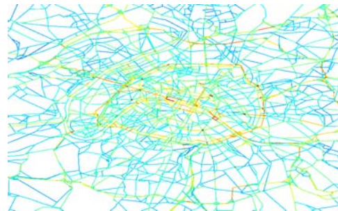
Figure 8 cold emission levels of CO for Paris metropolitan area between 9:00 a.m. and 12:00 noon
