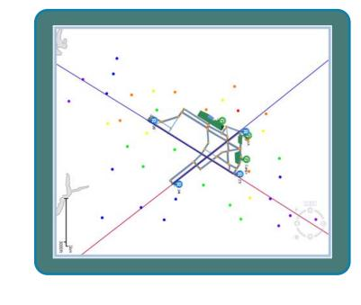
AEDT produces fuel burn, emissions, and noise. It can calculate and display results at the individual track segment level or aggregate the results up to various spatial and temporal resolutions (e.g. daily, monthly, or annual). AEDT has integrated GIS capabilities, including the ability to overlay demographic data or other map layers, produce plots, or export tabular data for customized reports and analyses.
