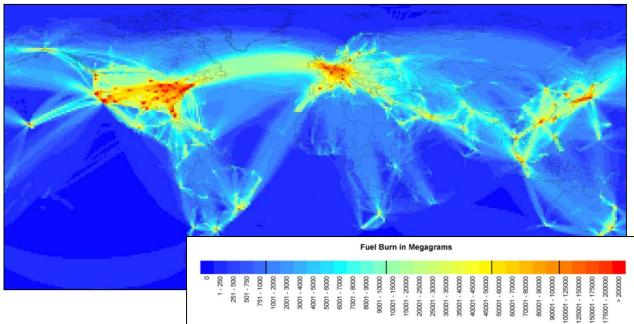
Global inventory of fuel consumption is a primary product of the application. Such results are easily transformed into emissions of CO<sub>2</sub>, criteria pollutants or HAPs.
